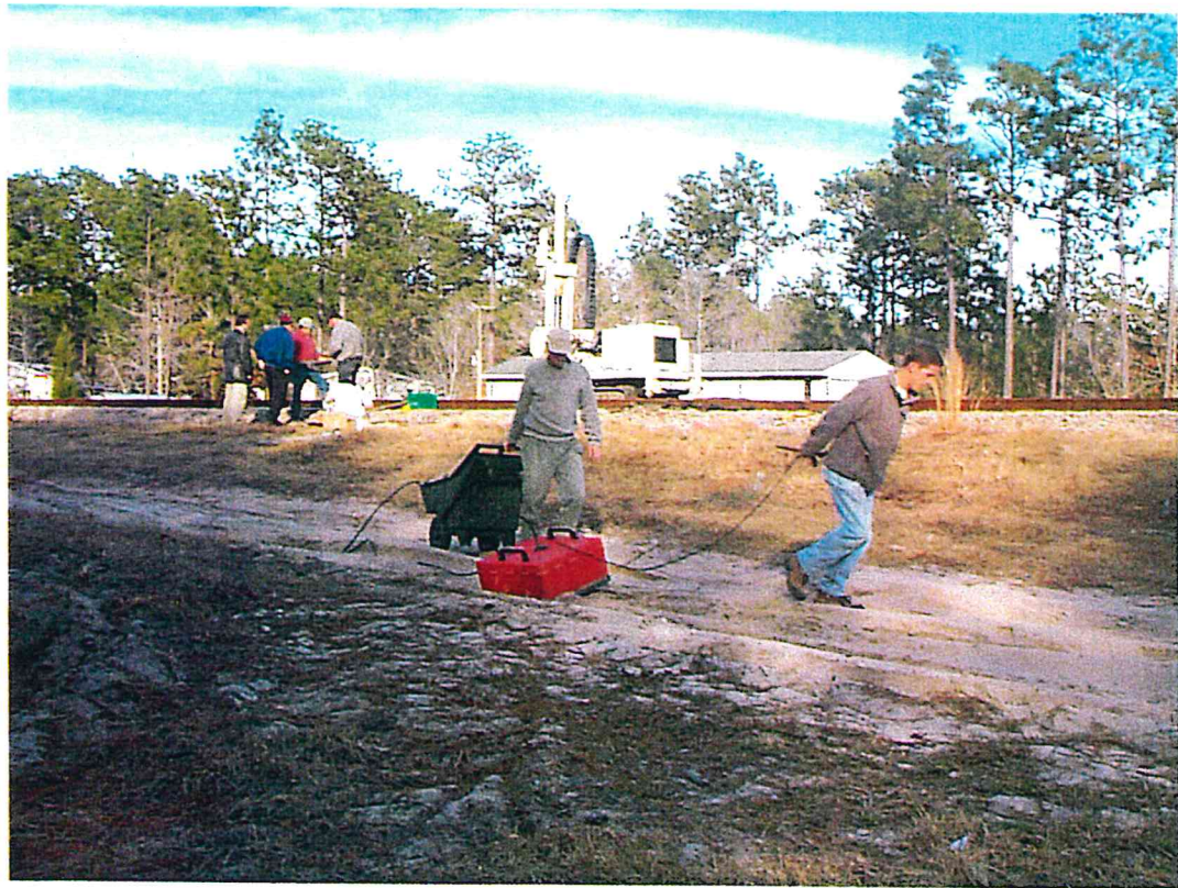
Photo 2. GPR Survey with Geoprobe in Background.
