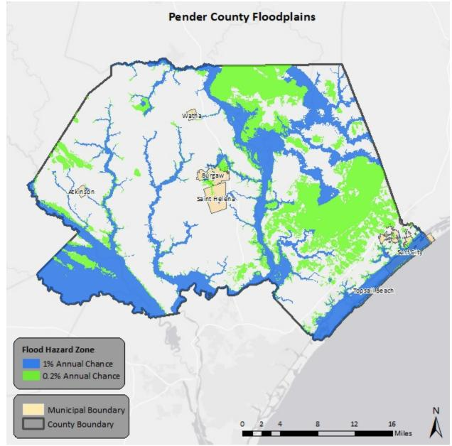
FIGURE 5.22: SPECIAL FLOOD HAZARD AREAS IN PENDER COUNTY
