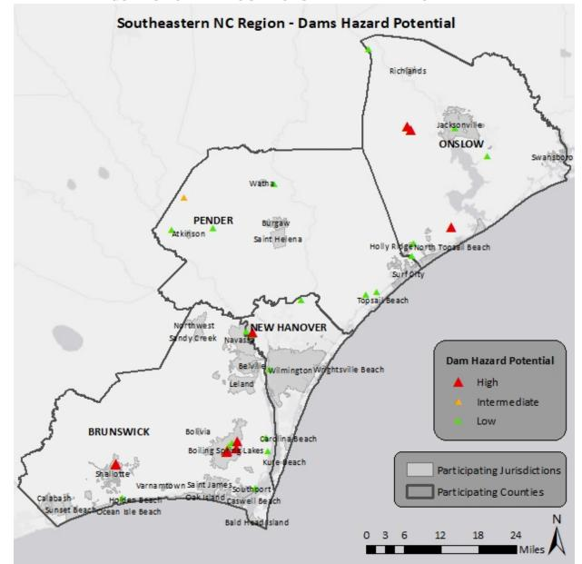
FIGURE 5.18: DAM LOCATIONS AND HAZARD POTENTIAL
