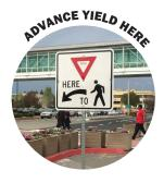
Advance Yield Here To Pedestrians signs are placed in advance of the marked crosswalk along with the stop line or yield line to alert drivers.
