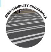
High visibility crosswalks are crosswalks marked with diagonal or longitudinal lines parallel to traffic flow, such as the ladder, continental or bar pair marking pattern.
